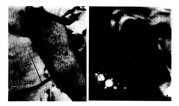
Figure 4. (a) Bright- and (b) dark-field TEM images of a small twin grain in a (110) grain matrix, having an irregular, lenticular shape. Dark-field image is obtained utilizing a primary twin reflection and extra, kinematical reflections shown circled.
